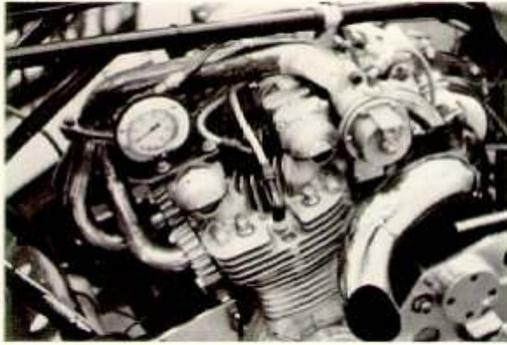
Fig.112 Drag bike turbo installation
