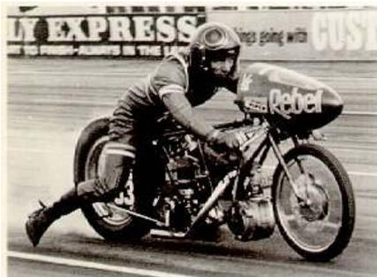
Fig.113 Positive drive blower on drag bike
