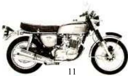
Fig.11 is a standard street Honda 750 four and Fig.12 is a full race version of the same model. The noticeable external differences in the engine preparations are to increase the VOLUMETRIC EFFICIENCY.
