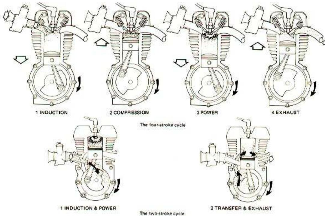
Two stroke or four stroke, one cylinder or sixteen, the conversion process is always carried out in the same way - by drawing in a mixture of fuel and air, compressing it, igniting it and using the resultant combustion to drive a piston or turbine down or round, and rotate a crank.
