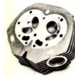
The mixture enters the cylinder head and is induced through the inlet valve into the combustion chamber. The way in which it enters the chamber is controlled by the
