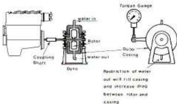
It uses a device like the torque - converter of an automatic transmission to do the job of the rope and drum and is running in a continuous flow of cooled water to absorb the heat.
