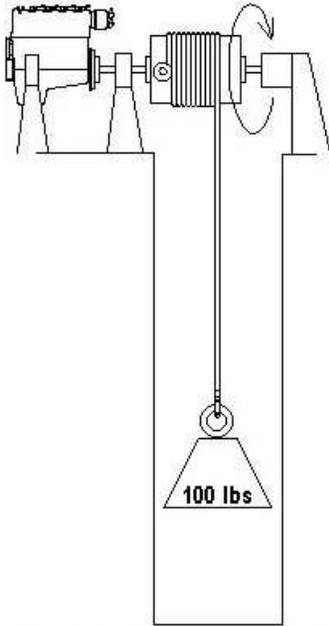
Imagine an engine sited at the top of a deep well turning a drum, which is four feet in diameter, i.e. 2 feet radius.
