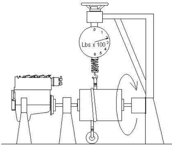
To understand the way in which the dynamometer works, imagine anchoring a spring balance to the ground, with a rope attached to the top eye and wrapped around a drum with a slipknot is tightened as the drum is rotating, the rope will be tensioned and the balance will extend to indicate this tension as a 'weight'. As the knot is further tightened, friction between rope and drum will slow the drum and its driving engine until, at 1000 R.P.M, the spring balance reads 100 lbs.
